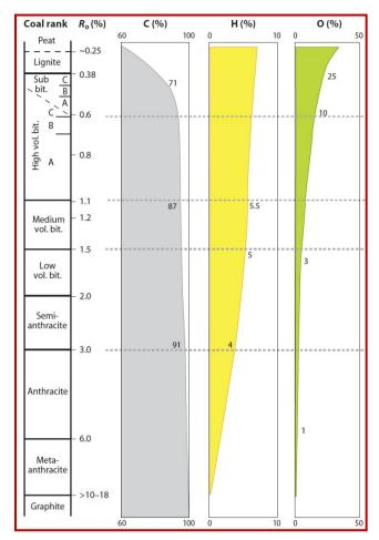
Figure 2. Changes in selected chemical properties of coal throughout coalification (Modified after Stach et al., 1982)
